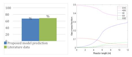
Fig. 2: Conversion of methaneFig. 3: Gas composition profile in multi-tubular reactor vs reactor length
