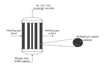
Fig. 1: Multi-tubular reactor with catalyst
