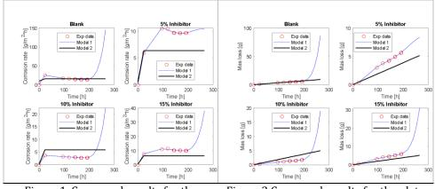
Figure 1. Compared results for the corrosion rate Figure 2 Compared results for the plate mass loss
